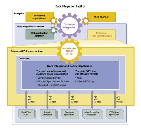
A Java application and toolkit, DIF enables integration of POS data to targeted destinations across the enterprise. DIF is installed on a 4690 POS controller and consists of a programmer's application programming interface (API) and a runtime process. These tools enable the following kinds of messaging:
