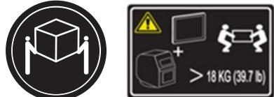
The weight of this part or unit is between 18 and 32 kg (39.7 and 70.5 lb). It takes two persons to safely lift this part or unit. (C009)
