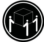
The weight of this part or unit is between 32 and 55 kg (70.5 and 121.2 lb). It takes three persons to safely lift this part or unit. (C010)
